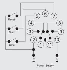
Note: The positions of the relay contacts are shown in the de-energised state.
